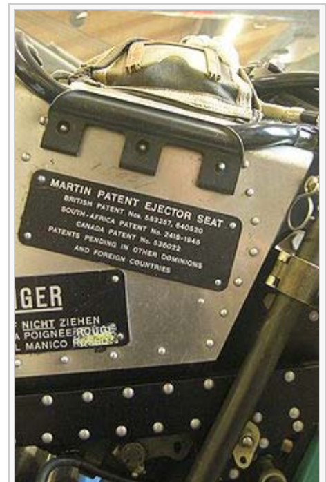
The plate of the Martin ejector seat of the military aircraft, stating that the design is covered by multiple patents in Britain, South Africa, Canada and "others". Dübendorf Museum of Military Aviation .
